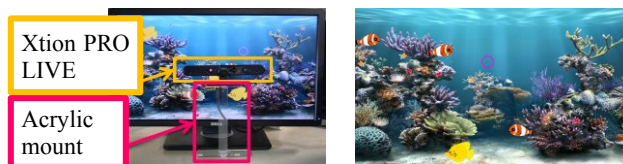
Figure 6: Left: Hardware layout of secondary system; Right: Screenshot of the revised second application.
