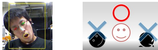
Figure 7: Left: robust recognition for rotation. Right: face orientation notifier (red circle: OK, blue cross: FAIL).
