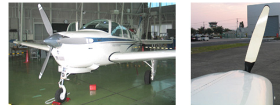
figure.4 Left: Bonanza A36, Right: Retro-reflective sheet applied to a blade (white area of the blade)
