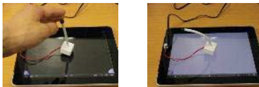
Figure 5 Detecting a touch event (left: immediately before touch; right: after a touch)
