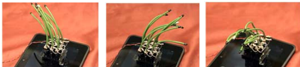
Figure 6 Multi-directional type of the hairytop interface
