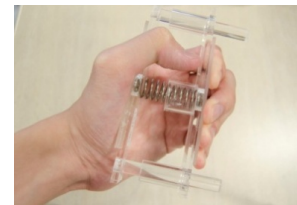
Figure 4. Physical Stimulus(PS) composed of a physical spring.
