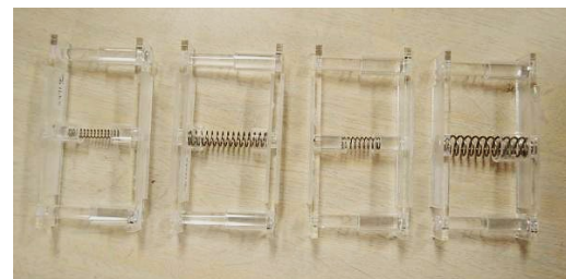
Figure 5. PSs installed with different springs ( k=0.471, 0.853, 1.197, 1.521 in order from left to right).
