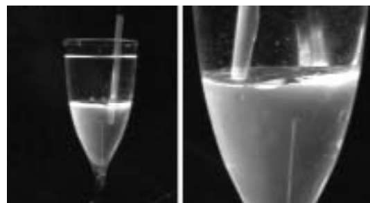
Figure 8 Touching the interface between oil and water (Left: normal tool penetrate the interface Right: the tool of the SmartTool stops at the interface)
