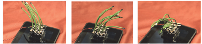
Fig. 13 The movement of the multi-directional type of the smart hair
